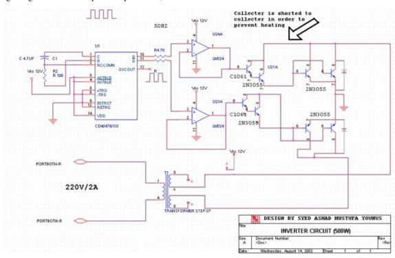
This circuit is generating a square wave of 50Hz through the 4047 IC, where the tansistors are amplifying the current. The transistors can be replaced by FETs to have lower power dissipation and faster switching. The driver circuit can be changed to have a modified sine-wave, as square wave is not good for many electric appliances. The below driver circuit example creates a modified sine waveform. The frequency and pulse width can be modified with R1 and R2.
