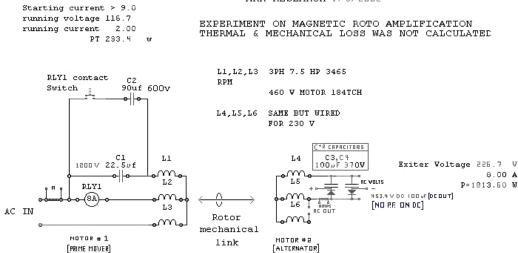
The second schematic is an RV looped system. There is one cross-phase cap to tune and keep the alt in semi-resonant state, and there are three coupling caps where again RF and POWER transformer rules apply.
